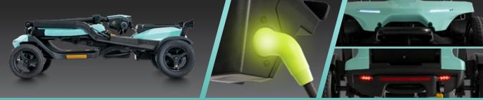
Folds to a depth of only 12" without having to remove the seat.
