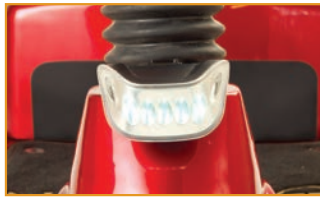
Angle adjustable LED headlight creates a wide path of bright light
